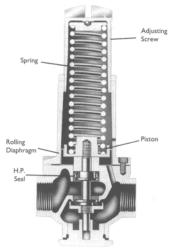
6. If necessary, reset the pressure by turning the Adjusting Screw and then checking the new dead end setting.
